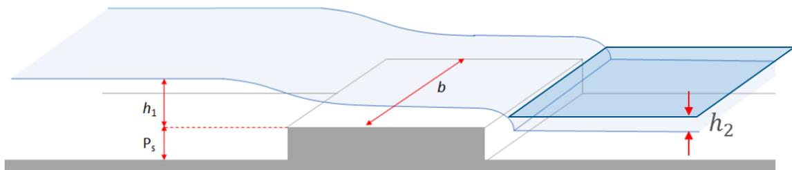
Weir parameters are entered via the properties structure block command as follows:
