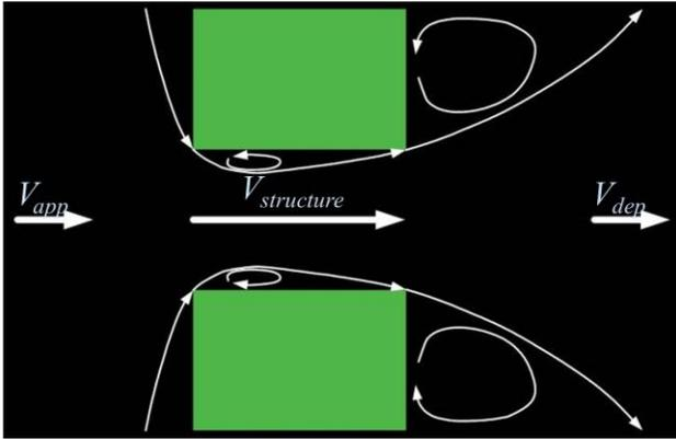
Entry and exit loss adjustment is switched on by default as set by the fourth entry of the culvert parameters command:
