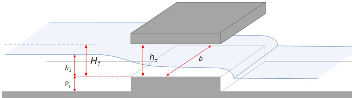
The default culvert\_critical\_hd is 99999, i.e. the upstream controlled flow regime is applied once the first condition is met. To adjust the depth threshold or to switch off inlet control for backward compatibility the culvert parameters can be set using the `Culvert Parameters ==` control file command (Note `Culvert Parameters ==` is not a structure block command), e.g. changing the first culvert parameter to 0. (metres or feet) switches off the inlet control regime:
