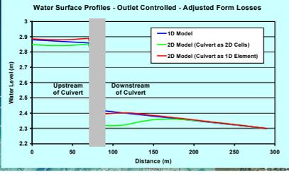
Water Surface Profiles - Outlet Controlled - Adjusted Form Losses
