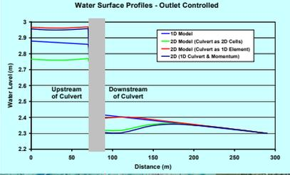
Water Surface Profiles - Outlet Controlled
