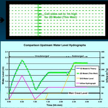
Cell sides set to 1m high for 2D Model (Thin Weir)
