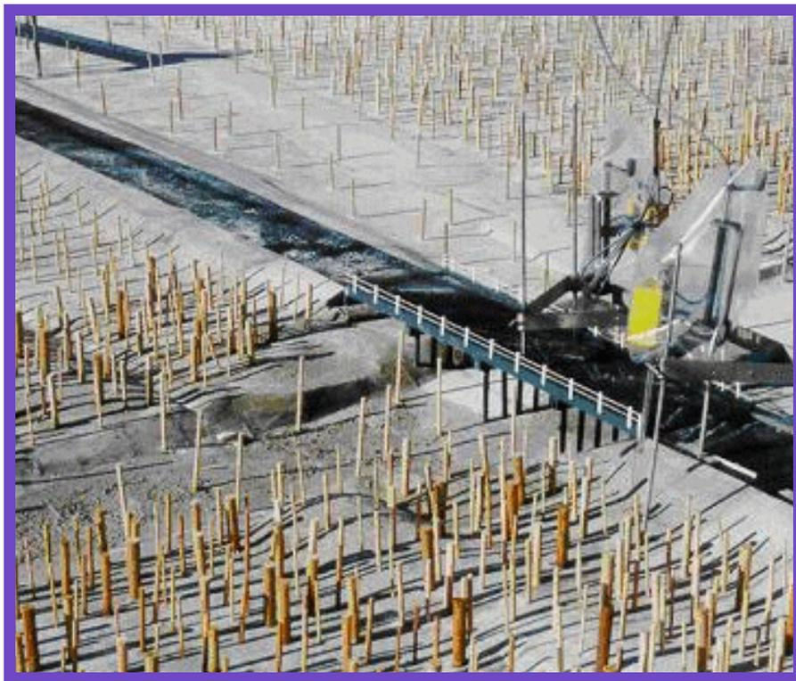
*Figure 1. Eudlo Creek Physical Model Showing Four Span Bridge*
