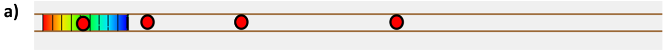
Figure 4 - Spatial figure of a plan view of the channel in which the dam break occurs. The coloured contour corresponds to the wedge of water before the gate is released, and each dot in the channel corresponds to the static location at which the data is taken over time. These points correspond to the locations at which the curves in Figure 3b are taken.
