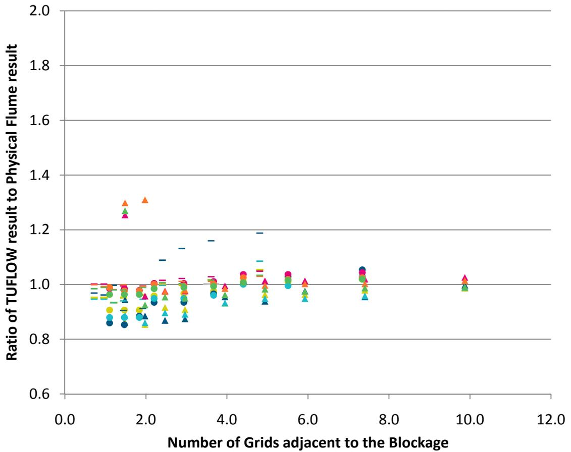
**Figure 4-7** Abutment Analysis – Influence of Grid: Blockage Ratio (Excluding 2 and 3 Foot Openings)
