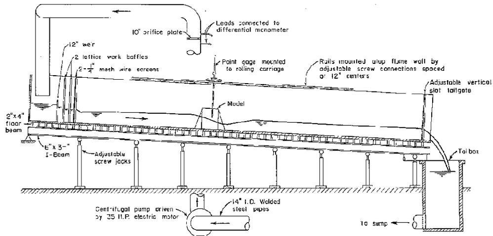
**Figure 3-1 The Physical Flume used by Liu et al (1957)**
