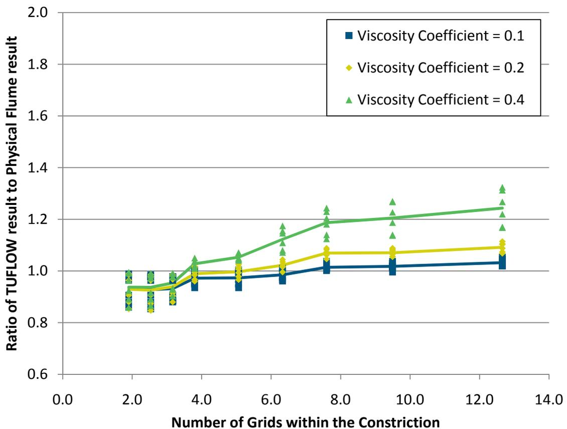
Figure 4-1 Influence of Viscosity Coefficient
