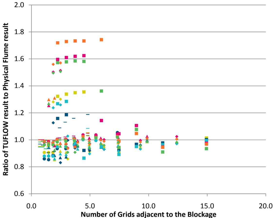
**Figure 4-6 Abutment Analysis – Influence of Grid: Blockage Ratio**
