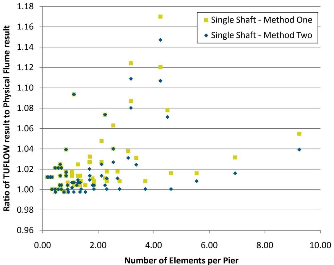
Figure 4-9 Pier Analysis – Single Shaft Piers
