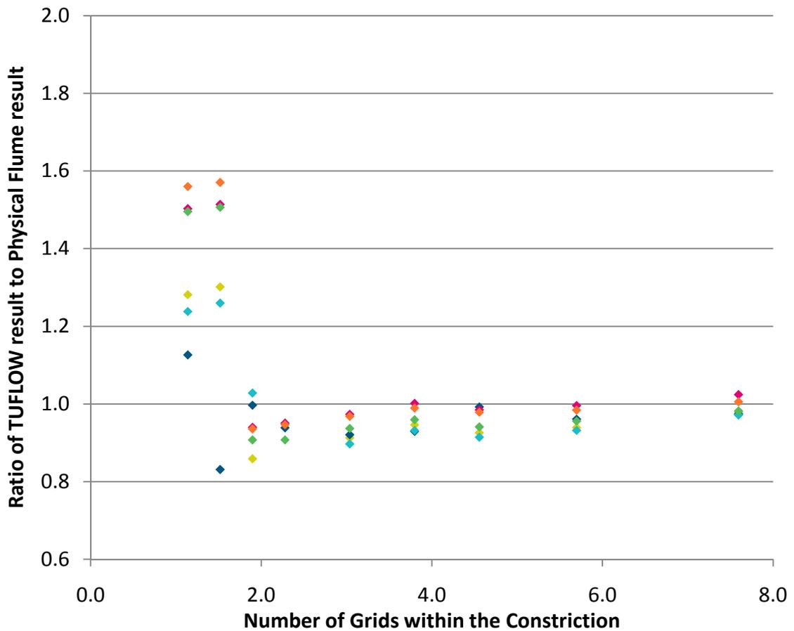
**Figure 4-3 Abutment Analysis – Influence of Grid: Constriction Ratio (3 Foot Opening)**
