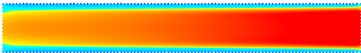
Flow separation along a dry oblique boundary without enhanced treatment of viscosity term
